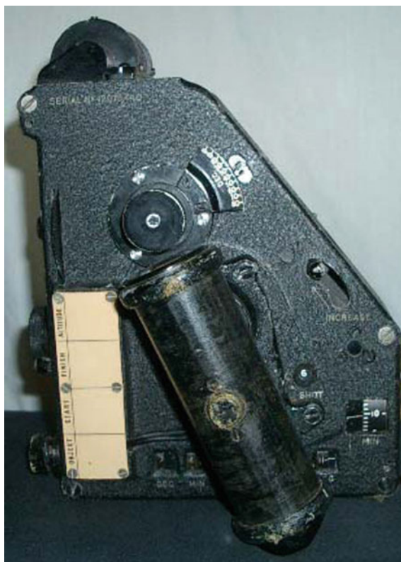
A RAF Mark IX Bubble Sextant courtesy of Military Autographs UK ( Image credit militaryautographs.com )
